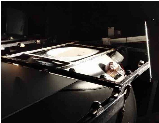
Fig. 4 Spectrophotometer with an Ulbricht sphere, 1 m in diameter, with a movable arm enabling angular measurement
